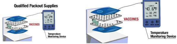
**Alt text:** Qualified Packout Supplies for vaccine transport: Vaccines, coolant and insulating materials, with digital data logger to monitor temperature.
